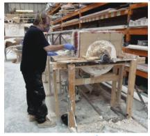
Pictured above is the manufacture of a fluted column master. The columns are to be made in Scagliola. Mike Berry a Scagliola craftsman is pictured making the fibreglass mould casing.
