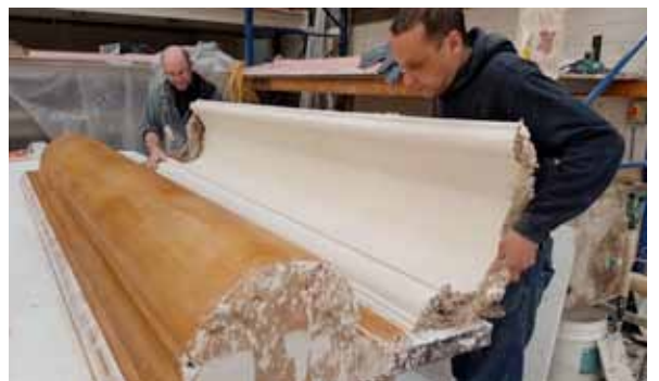
Hayles and Howe craftsman, Justin Anderson is pictured above and below with workshop foreman Martin Henry manufacturing a large panel coving to match the existing panel surround, as pictured left.
