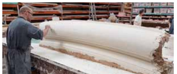
Hayles and Howe craftsman, Justin Anderson is pictured above and below with workshop foreman Martin Henry manufacturing a large panel coving to match the existing panel surround, as pictured left.
